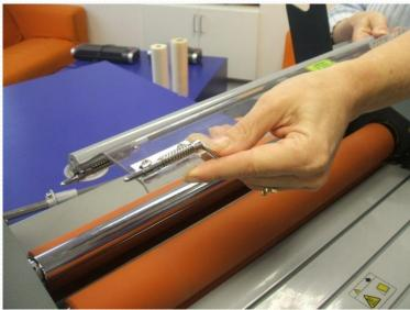
Carefully remove the feed tray by retracting interlock bolt
