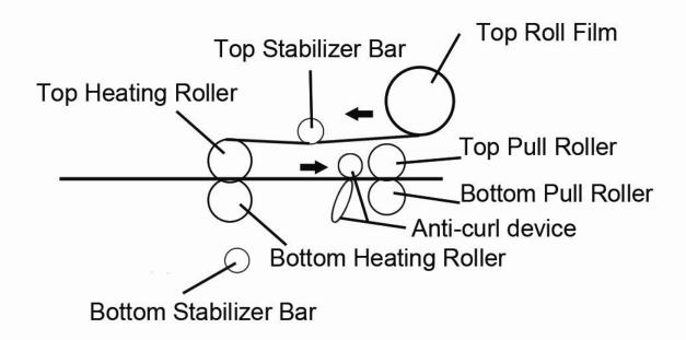
Thread film from top mandrel down under top idler bar and over top laminating roller surface as shown (ensure film is loaded with adhesive side up)
