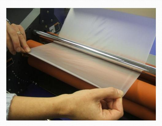
Lift top roller by turning roller pressure handle anti-clockwise.
