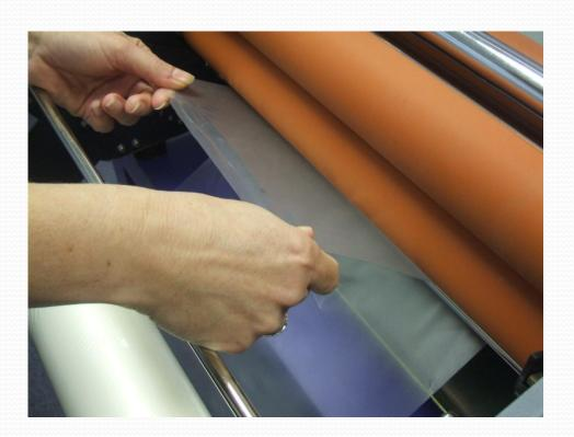
Bring top film down under idler bar and web the films together as shown overlapping the top & bottom film by several inches.
