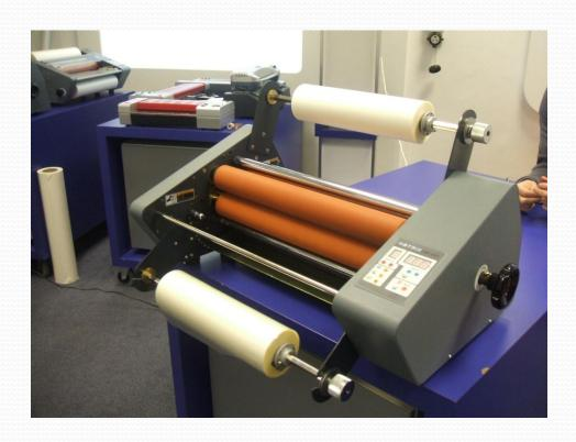
Select the 'BOTH HEAT' setting on the heater switch on the back of the machine.
