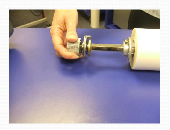
Refit top mandrel complete with film as shown.
