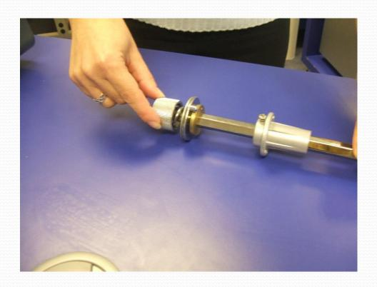
• Remove all components (tension handle, spring, tension plates and bearing) lay the parts out in order (as shown) so they can be easily refitted in the correct order.
