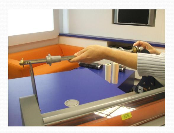
Completely unscrew the tension handle on the removed mandrel.
