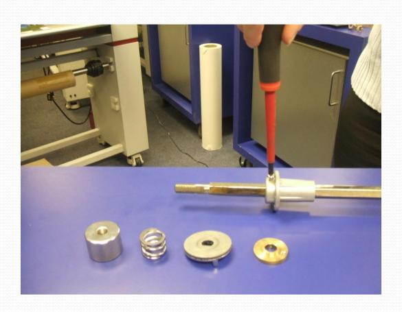
Load the film onto the mandrel and make sure it is loaded with the film coming off the bottom of the roll with the adhesive side up. Tighten the screw back up with a screwdriver.
