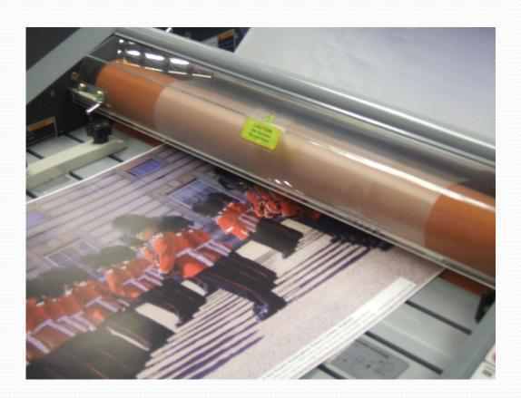
Press the 'HOT' button and dial in the desired temperature using the 'TEMP SET' switches. Ensure rollers are lifted whilst the machine is heating up.
