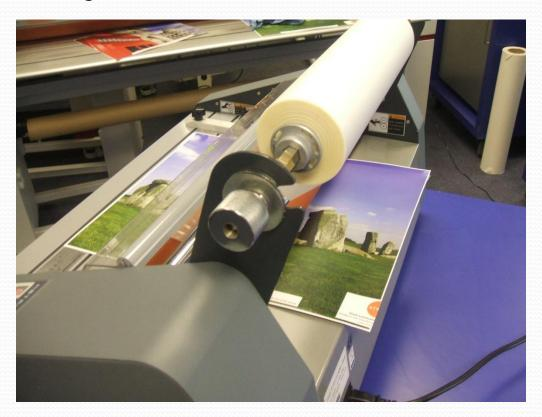
• When single side laminating ensure documents slightly overlap as shown. Leave one edge outside of the laminating film giving you clean edges for guillotining.
