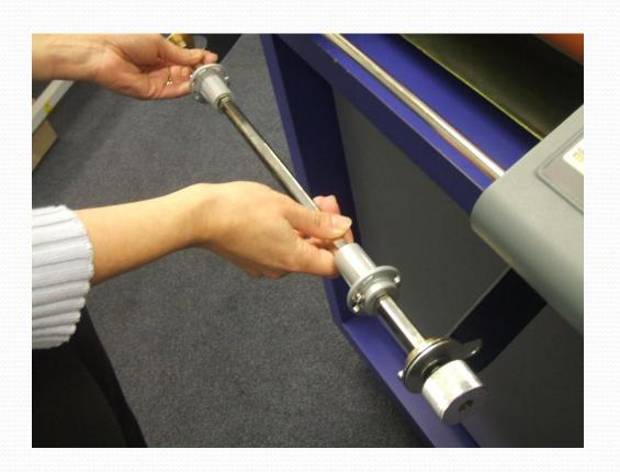
Whilst film and bottom mandrel are removed select the anti-curl bar to setting '0'
