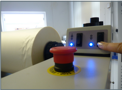
21. Press pull roller switch. Roller will lower and light should illuminate.
