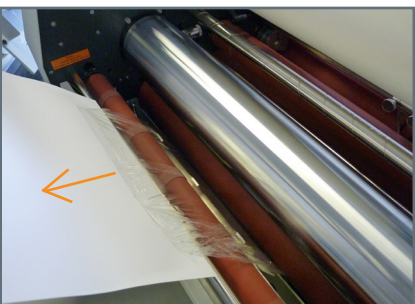
14. Pull fed card back towards the front of the system as shown.
