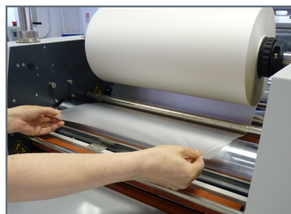
14. Run the film under the idler bar and drape over the steel laminating roller.
