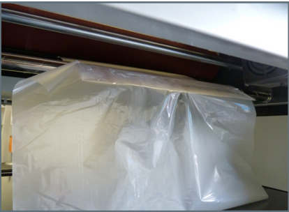
13. Tape bottom film to the feed card.
