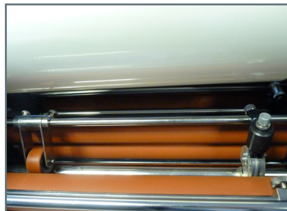
25. Set the guide wheel to the opposite side of the sheet from the perforation wheel.
