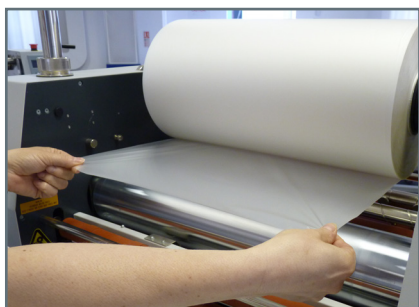
10. Ensure film feeds from the bottom of the roll.
