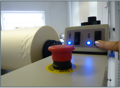
19. Press pull roller switch on pneumatic control unit. Roller will lower and light should illuminate.
