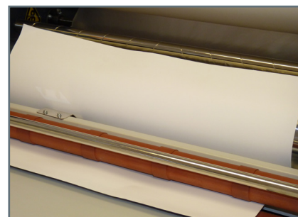
15. Press second set-up print onto the film.
