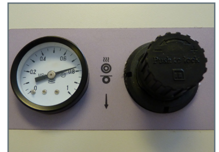
27. Adjust laminating roller pressure as required. Suggested pressure between 6-8 bar.
