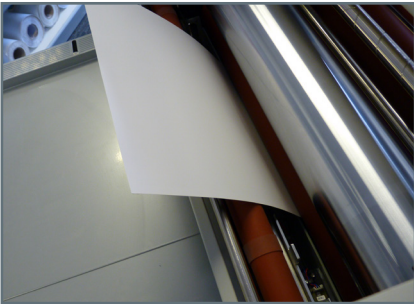
12. Push a feeder card down around the bottom laminating roller.
