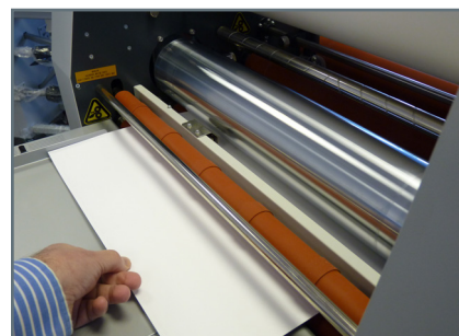
12. Press rubber roller to drop gate and slide in plain print, ensure it goes through anti-curl device and into pull rollers.
