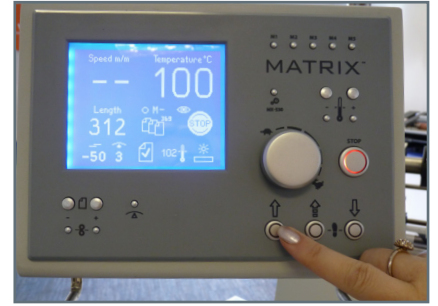
24. Push the forward button and select slow speed to load.
