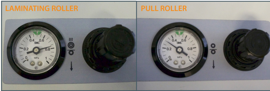
19. Laminating roller full pressure is 8 bar. Pull roller between 3-4. Please note these are guides only and for thinner stocks the laminating roller pressure may need to be decreased.
