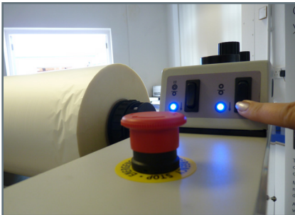
19. Press pull roller switch. Roller will lower and light should illuminate.
