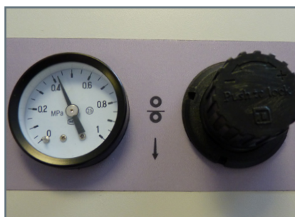
28. Adjust pull roller as required. Suggested pressure between 3-5 bar.
