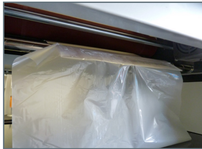
13. Tape bottom film to the feed card.
