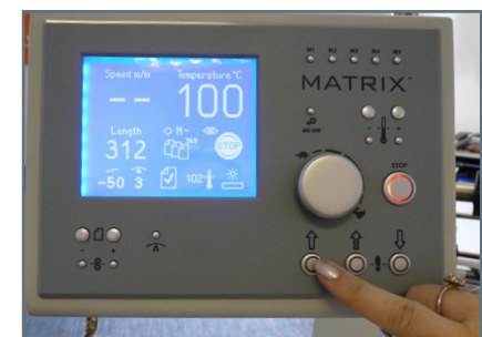
26. Press the forward button and select a slow speed (0.5-2.0m/m) to load.
