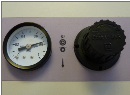
25. Adjust laminating roller pressure as required. Suggested pressure between 6-8 bar.
